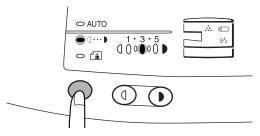
Use the light ((a)) and dark ((b)) keys to adjust the exposure level. If exposure level 2 is selected, the two left-handmost indicators for that level will light up simultaneously. Also, if level 4 is selected, the two right-handmost indicators for that level will light up simultaneously.
